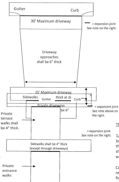
1/2" expansion joints shall be used at these two locations and shall completely separate all concrete in the driveway approach and driveway from the concrete in the sidewalk and in the curb including the rolled-up portion of the curb and driveway approach.
